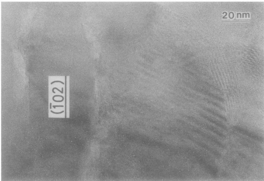
FIG. 7. Electron micrograph of the area where the superstructure is not formed in spite of heating.
